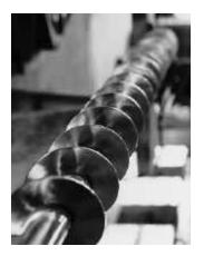
stainless steel (304, 316, 309, 310, etc.), hastelloy, inconel, AR steel etc. If needed, we will polish to a #4 finish with continuous welds to CEMA IV, a Dairy or pharmaceutical finish. Our design and manufacturing have passed USDA inspection. When needed we will assist in the proper selection of specialty hardfacing and apply as required to combat abrasion.
